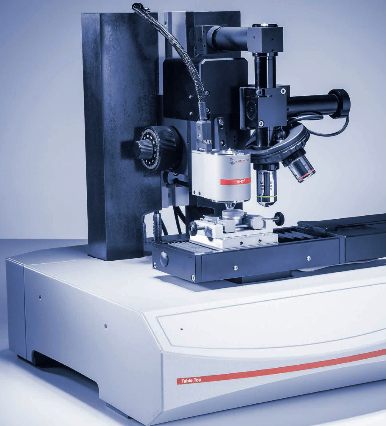
An example of sinus mode (dynamic mechanical analysis, DMA) performed by a nanoindentation tester.
