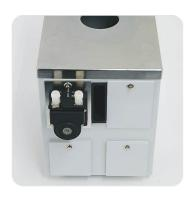
FlexyCUBE operating with a single peristaltic pump, used for volumetric dosage
