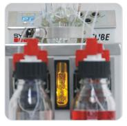
Convenient reactor handling; simply place the reactor assembly into the receptacle provided
