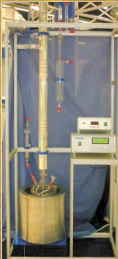
The versatile PILODIST 104 distillation apparatus achieves a high separation efficiency of up to 100 theoretical plates.
