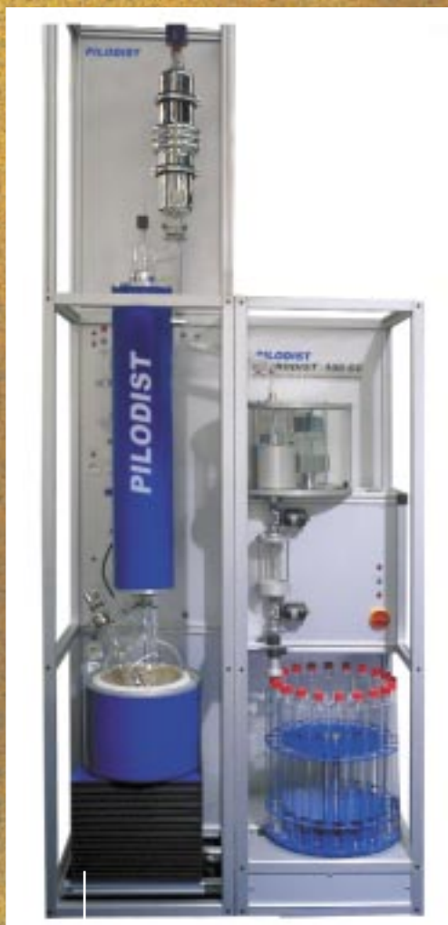
Particularly user-friendly distillation of crude oils according to ASTM D 2892 with the Petrodist 100 CC.
