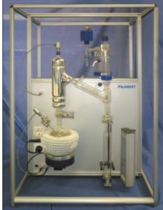
Petrodist 300 CC examined samples under vacuum according to ASTM D 1160.
