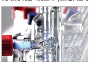
worldwide reputation for top quality and conformity to test specifications. All glass products are produced from borosilicate glass which is resistant to high temperatures and the most suitable raw material for our systems.
