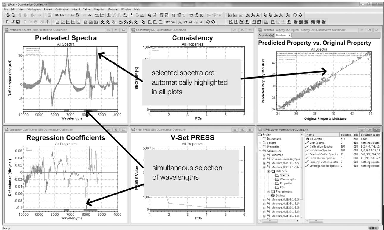
Easy selection of data sets (e.g. spectra, properties, wavelength, principal components) in graphic and table view. Live update of selected data within all corresponding plots and tables. Broad variety of visualization tools, like overview or dependency plots (e.g. data versus time, creator, instrument, property). Rapid calculations of large data sets.
