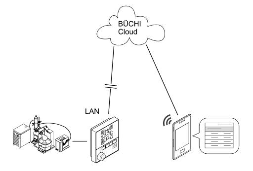
BUCHI Connect Scenario using distillation system, using smartphone, cloud and server.
