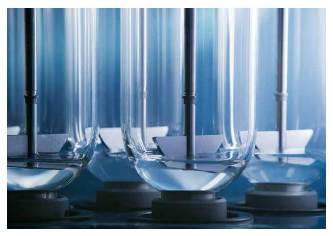
→ Simultaneous media dispensing into the vessels through the hemispheric valves
